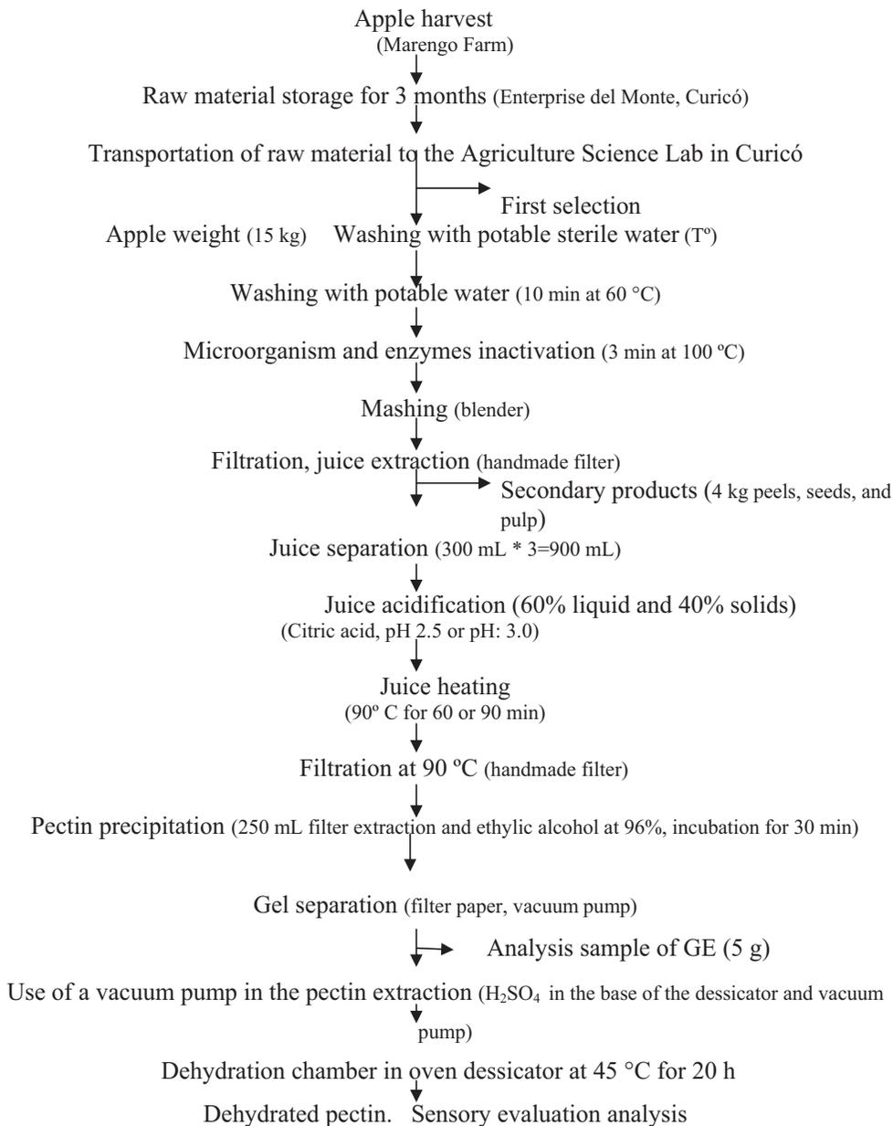
**Figure 1.** Flow sheet of pectin extraction.
