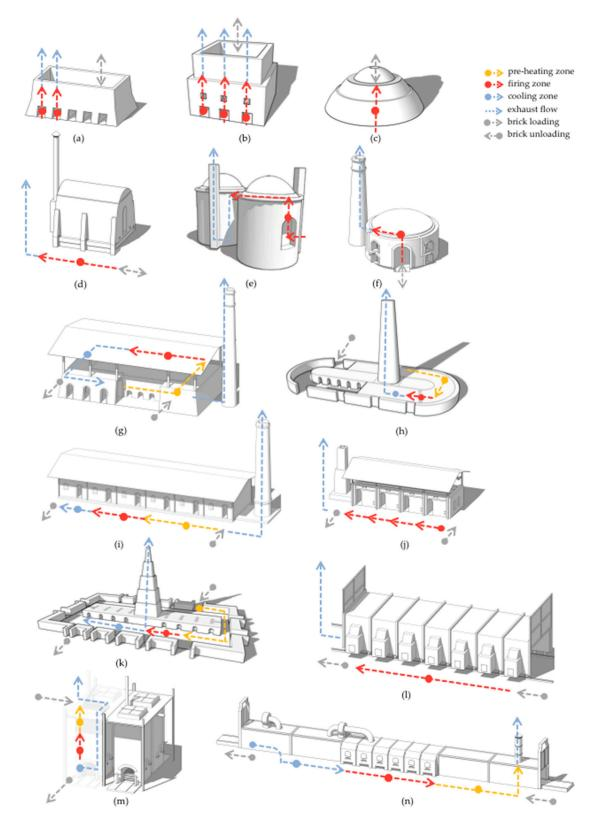
Figure 5. Drawings of the intermittent and continuous ovens. The arrows indicate the flow of brick loads and gas flow. (a) Open kiln without fixed walls (rectangular), (b) open kiln with fixed walls, (c) open kiln without fixed walls (cylindrical), (d) down-draught, (e) MK, (f) dome, (g) Hoffman, (h) Bull's Trench, (i) Cedan, (j) multi-chambers, (k) zigzag, (l) mobile-modular, (m) vertical shaft and (n) tunnel.
